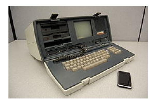
An Osborne Executive (\$1500) portable computer, from 1982, and an iPhone, released 2007. The Executive weighs 100 times as much, cost 10 times as much, and has 100 times less processing power than the iPhone (.
